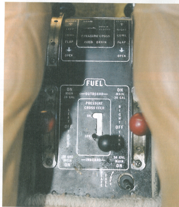
ABOVE: 'Juliet Whisky's' panel remains almost entirely as it was in 1972, excellent original features include ergonomically-shaped throttle, propeller pitch and mixture levers LEFT: tucked between the seats, the fuel tank and cross feed selectors, and (top of image) cowl flap controls BELOW: overhead elevator trim crank/rudder trim knob and lighting controls
