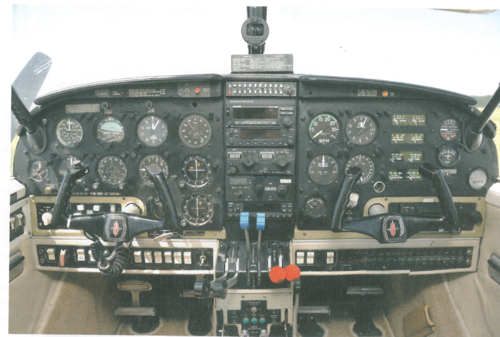
ABOVE: 'Juliet Whisky's' panel remains almost entirely as it was in 1972, excellent original features include ergonomically-shaped throttle, propeller pitch and mixture levers LEFT: tucked between the seats, the fuel tank and cross feed selectors, and (top of image) cowl flap controls BELOW: overhead elevator trim crank/rudder trim knob and lighting controls
