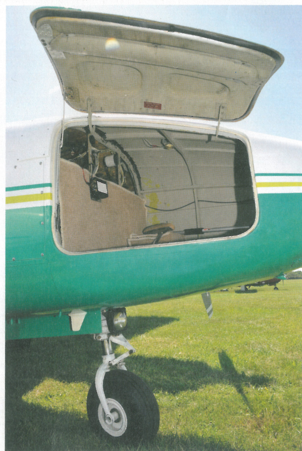
ABOVE: there's plenty of space for baggage, sensibly distributed between space in the nose... BELOW: ... and the neatly trimmed compartment behind the cabin (note the Y-shaped cluster of frame tubes) RIGHT: in the Piper tradition and interest of structural integrity, there's just the one cabin door
