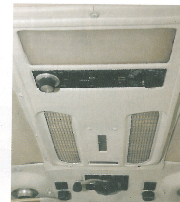
ABOVE: 'Juliet Whisky's' panel remains almost entirely as it was in 1972, excellent original features include ergonomically-shaped throttle, propeller pitch and mixture levers LEFT: tucked between the seats, the fuel tank and cross feed selectors, and (top of image) cowl flap controls BELOW: overhead elevator trim crank/rudder trim knob and lighting controls
