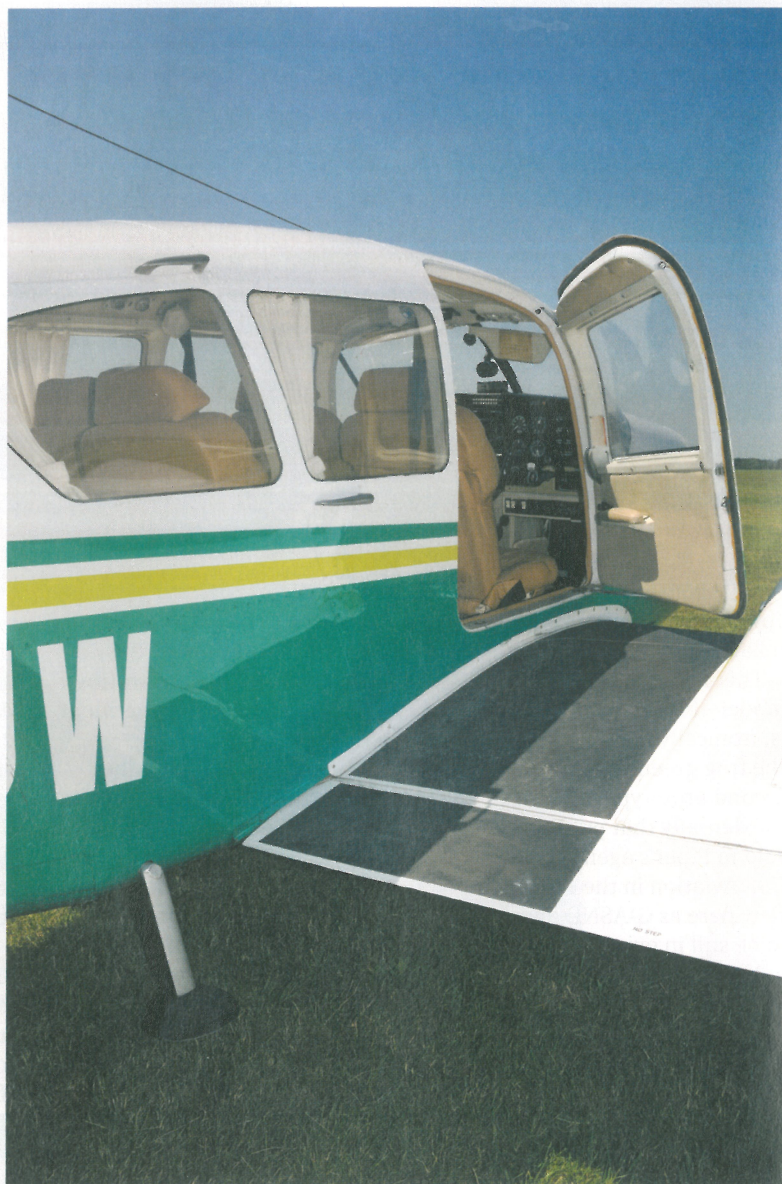
ABOVE: there's plenty of space for baggage, sensibly distributed between space in the nose... BELOW: ... and the neatly trimmed compartment behind the cabin (note the Y-shaped cluster of frame tubes) RIGHT: in the Piper tradition and interest of structural integrity, there's just the one cabin door
