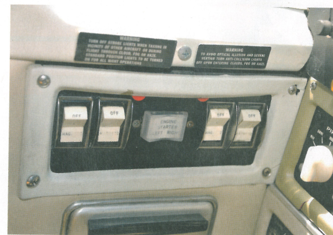
Starter and mag switches are located on the port fuselage wall
